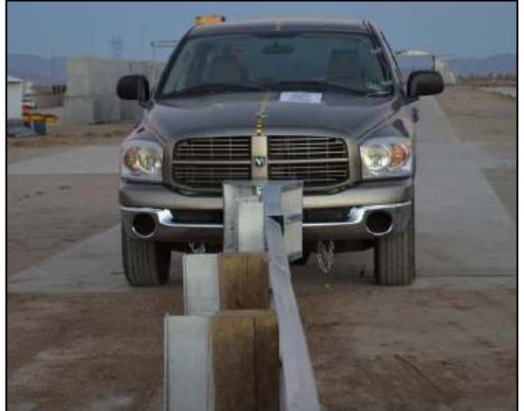
MASH Test 3-33 Set-Up (2270P at 100km/h and 5°)
