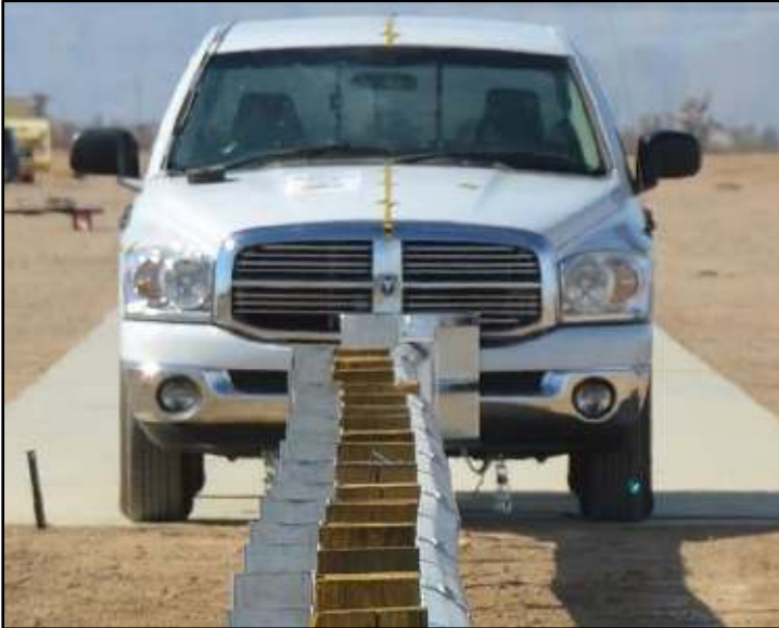
MASH Test 3-31 Set-Up (2270P at 100km/h and 0°)
