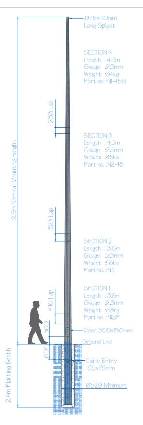
Steelgal NZ Limited Product : NOMINAL 12.9m GROUND PLANT OCTAGONAL FLOODLIGHT POLE 8 Trugood Drive Drawing No. : OT-FLD-129-P-1 Standards Pole Design AS 4676 / AS 1170.2 Sect'n4 / NZS 4203 East Tamaki Drawing size: A4
