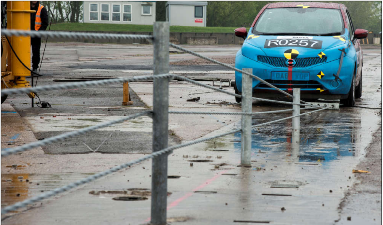
Figure 13: Cable Weave at Terminal
